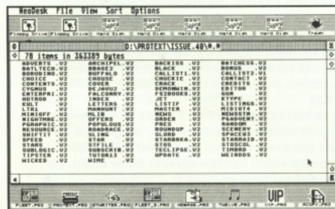
Here files are shown as text with the details of size, date and time removed. Neodesk fits as many files as it can in the window, according to the amount of information you have selected. In this instance there are 78 files in full view. These can be quickly switched to single column if it is easier to view them that way.
